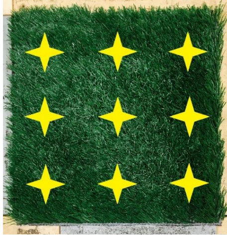
Figure 1. Locations for infill height measurements of the testing turf piece.
